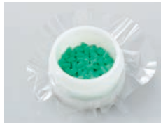
Cover the bottom of the cell with film and add the sample.
