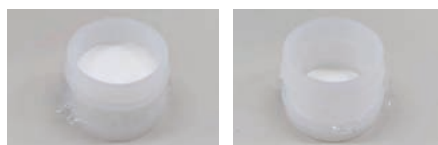
Sufficient amount (3.0 g) Small amount (0.5 g) Appearance of cellulose powder sample (using sample container)
