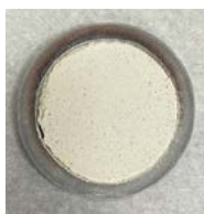
Sample appearance (Pressure molding with a total pressure of 250 kN for 30 sec)
