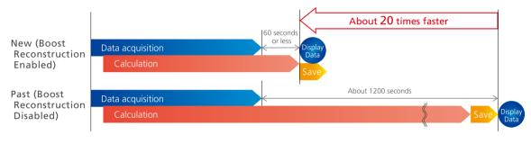
\* The above shooting conditions are as follows: clear mode, full scan, 2400 View, 1500 slices, image reconstruction size 2048 × 2048. \* Since Boost Reconstruction Function is a speed-specific image computation technology, it may affect the quality of cross-section images
