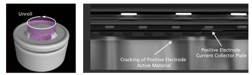
VR Image (Unrolled the Purple Cylinder) Unrolled Cylinder Cross-Sectional Image of Cathode Active Materials
